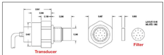
A typical sensor or transducer application of a planar filter cap
