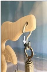
9. Suspend the spring using the 'S'-hook.
