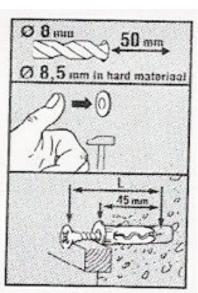
Place the wall plate over the holes. Screw the large screw bolts through the plate and into the plugs Look behind the plate to 'aim' for the plugs. When you are certain all 6 screwbolts are aimed correctly for the plug holes, take the wall plate down.
