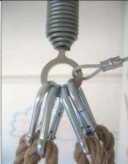
10. Now, attach the cradle using the 4 (small) carbine hooks.
