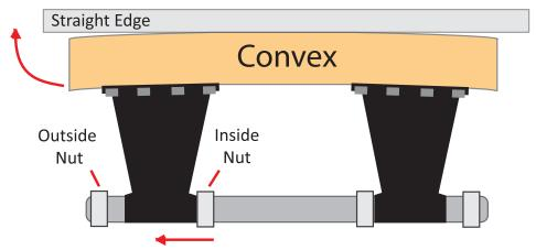
If the playfield is CONCAVE the bottom of the straight edge will be touching each edge of the playfield surface but not in the center. This should allow for the corner of a piece of paper to slide under the center of straight edge for approximately 3". If the playfield has an excessive concave shape, adjustments opposite the above for convex should be made as shown below.
