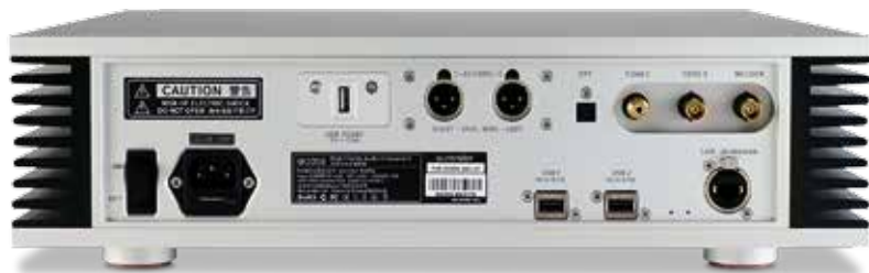
ABOVE: An isolated Gigabit Ethernet port [lower right] is joined by two USB-A 3.0 hubs for outboard drives and an external word clock input. Outputs are on USB-A 2.0 (384kHz/32-bit; DSD512), Dual-AES (DSD128 over DoP) and coax/opt (192kHz/24-bit)
