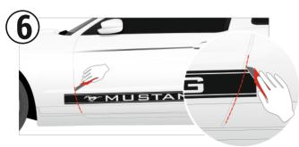
Cut unnecessary part of decal at the adjacent sing of element as showen on pic. Use Precision-Tip Vinyl Trimming Knife ties.
