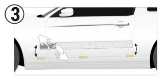
Partially remove the backing from the application tape/decal about 1/4-1/2 way.
