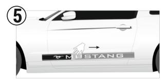
Carefully and slowly remove the application tape, pulling it off at the top corner at a 45 degree angle. If any air bubbles remain, they will usually disappear after a few weeks.
