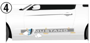
Once aligned, firmly press your hand down the application tape while removing more of the backing at the same time, slowly working your way down the decal. Use the included vinyl squeegee to firmly squeegee the application tape, working out any air bubbles from behind the vinyl. The vinyl is now bonding to the vehicle surface.
