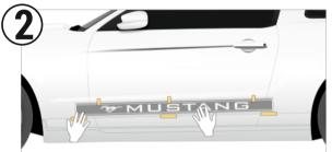
Hold vinyl graphic up to vehicle to check proper alignment and fitment. If you are installing the graphic over a vehicle seam, such as in the case with stripe kits, now is a good time to make cuts at the appropriate spots, ensuring that you leave an inch or so of extra vinyl material on each end to tuck into the vehicle seam.
