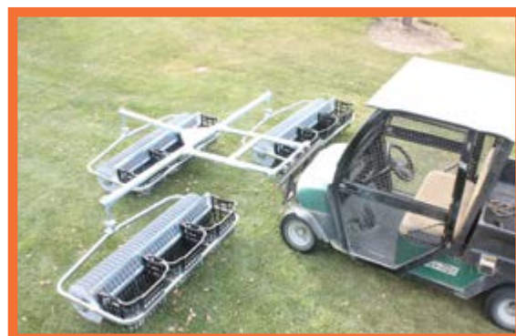
High Visibility Design All 3-Gangs sit in front of the driver, eliminating the “wings” on both sides of the driver that are typical on a 5-gang.
