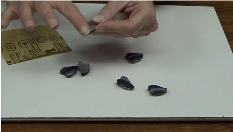
Finger test for smoothness. It's up to you to continue sanding with finer grits. I find it not necessary once the DeepShine has been applied.
