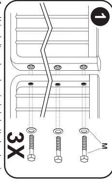
1. Using bolts and washers included, attach extension to hinge side of gate.
