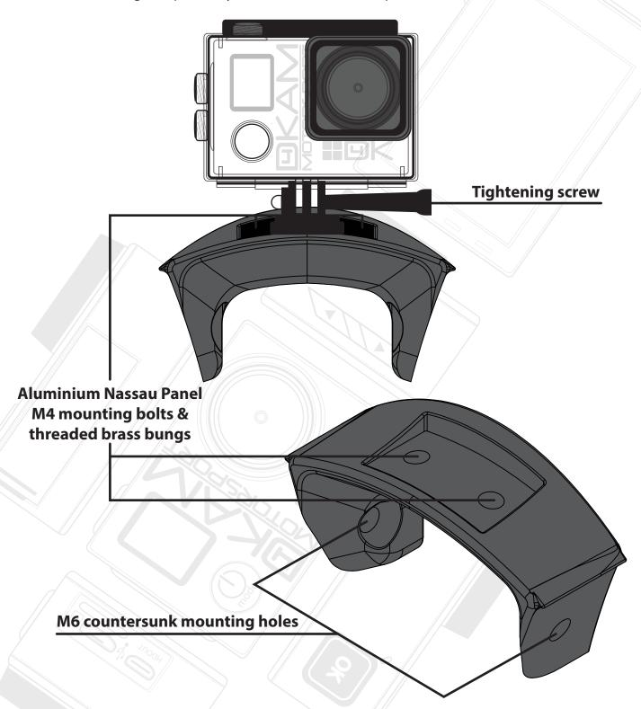
First align mount appropriately in accordance with regulating authority guidelines. With a scribe or small nail mark countersunk mounting holes onto Aero Nassau Panel and pre-drill to suit mounting bolt either M5 or M6 countersunk bolt. Be sure to use a washer and locknut or similar for affixing to the back of the bolt. NOTE: Do not overtighten the mount. Once the mount is fixed securely fit the camera and position accordingly being sure to do up the tightening bolt adequately.
