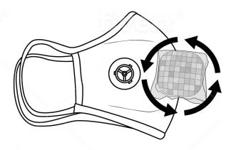
**Step 2:** Twist the "2.0 electric air valve" 'counter-clockwise' which will detach from the air valve's rim of the mask. Process shown on the photo.
