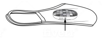
**Step 6:** Turn on the switch of the "2.0 electric air value" as shown. Then wear the mask.
