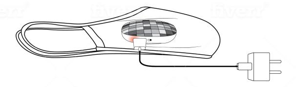
Plug the Micro USB cable in the micro-port OF THE "2.0 Electric air valve". Plug the other end into a USB port on your computer or other USB charging device. Typical charge time on an empty battery takes 1 hour.
