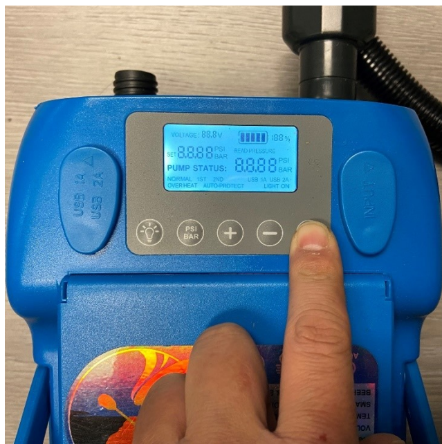
One Key Operate - Power ON & OFF, Pump START & STOP
