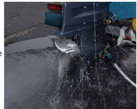
**NOTE** - Parsun outboards are water cooled. Running your outboard without an adequate source of cooling water will result in severe damage to the motor.
