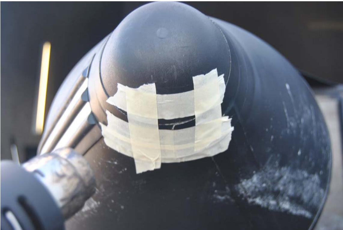
Before you start the repair, keep the boat chamber just inflated but soft. If you will use the electric pump, you may not read any pressure from the screen. So we can inject the thin glue from outside of seam leaking spot.
