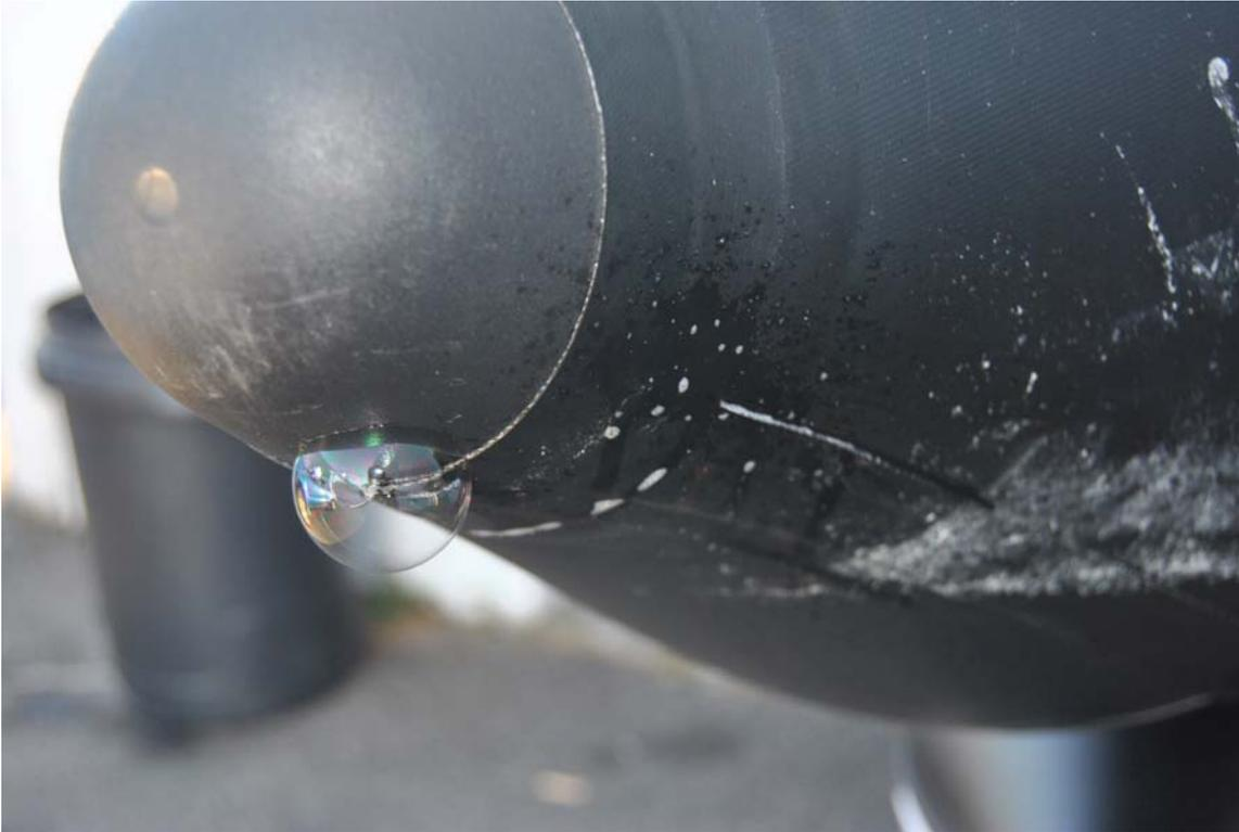
Tape or mark down the leaking location. Inflatable the boat to 3.6 PSI (25Kpa) and leave it dry for 24 hours. Air leaking will help the leaking spot dry fast. You can use heat gun or hair dry to speed it up.
