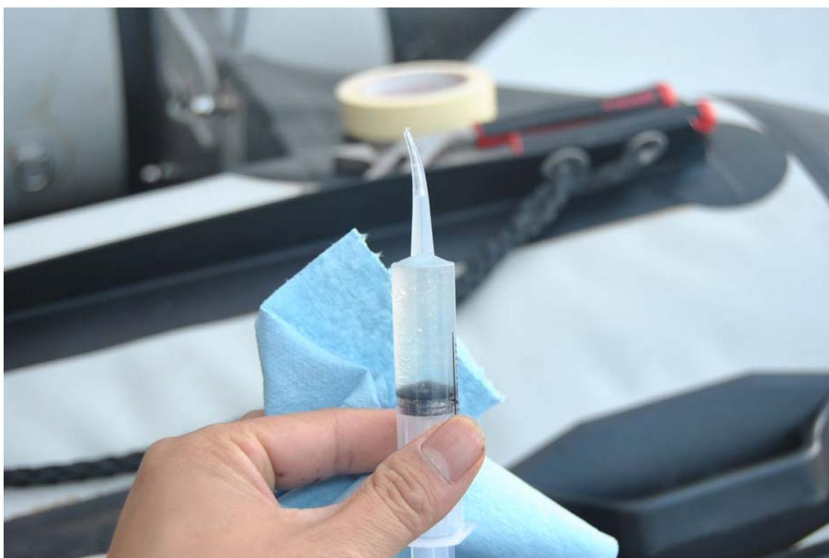
Inject the glue from the leaking spot.
