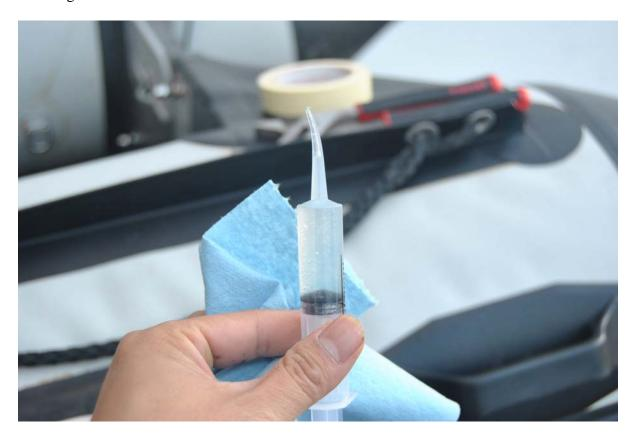
Inject the glue from the leaking spot.
