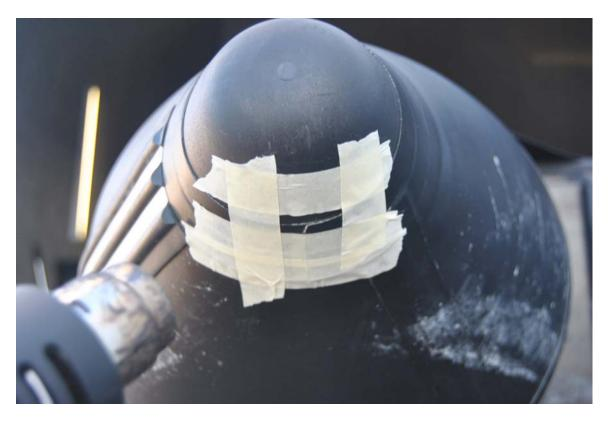
Before you start the repair, keep the boat chamber just inflated but soft. If you will use the electric pump, you may not read any pressure from the screen. So we can inject the thin glue from outside of seam leaking spot.
