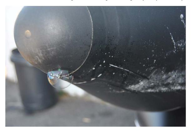
Tape or mark down the leaking location. Inflatable the boat to 3.6 PSI (25Kpa) and leave it dry for 24 hours. Air leaking will help the leaking spot dry fast. You can use heat gun or hair dry to speed it up.
