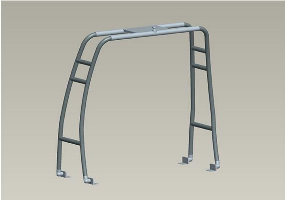
Step8: Assemble the tow eye on the top section, check if it is just at the center of the tower. Go over the whole tower and make sure all feet are connected without problem. Now you can drill the holes through the top section bar and connect the horizontal arms with 8x long bolts and nuts.
