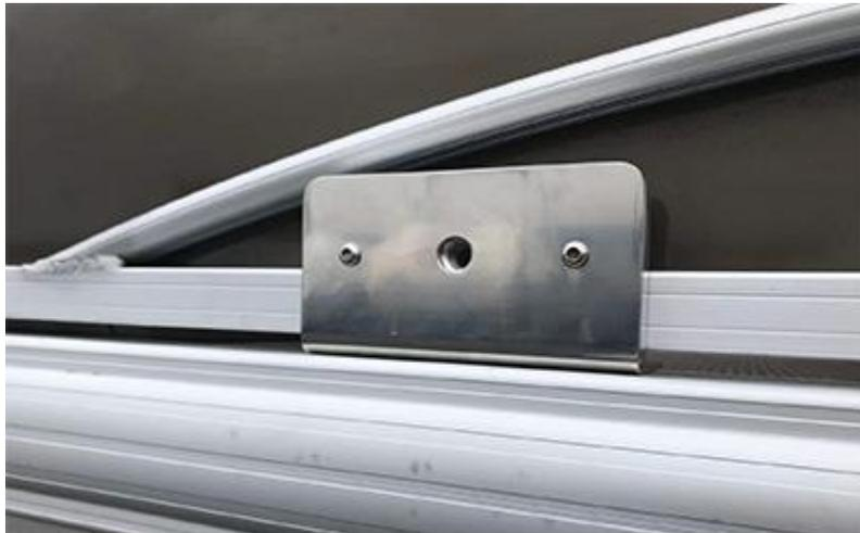
**Step3:** Measure the width outside to outside, and check if your dimension is between 78in-105in. If less than 78in, you may cut the horizontal arms to get a narrower tower. If above 105in, you may have to contact us to order a longer H top section.
