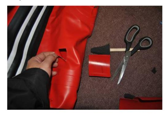
Draw a damage draft on the patch; make sure all edges of the patch are over 1 inch to the cut line (Min half inch).
