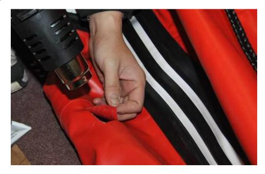
STEP5: Put the patch into the chamber through the cut
