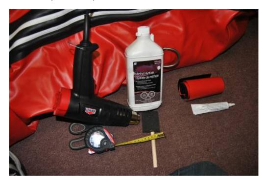
STEP 1: Proper clear up the Repair Area, if the cut is over ½ inch, the repair patches should be from inside and outside.
