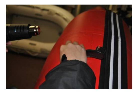
Stay the boat indoor for at least 5 Days to let the glue dry, don't pack the boat or deflate the chamber in this period. It may cause chamber stick together. Chamber is only inflated to 1 PSI. You can re-inflate the chamber after 24 hour to change the air inside. It will be better for the glue drying out.
