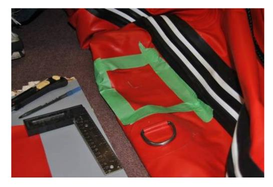
Inflatable the boat and Paint the glue on both surfaces. Give extra glue if not enough; make sure the outside patch can have well contact on the chamber.
