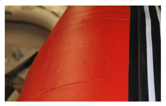
If you can't apply the outside patch in some case, using marine sealant from West Marine or Home Depot to seal the cut seam will be the 2<sup>nd</sup> solution.
