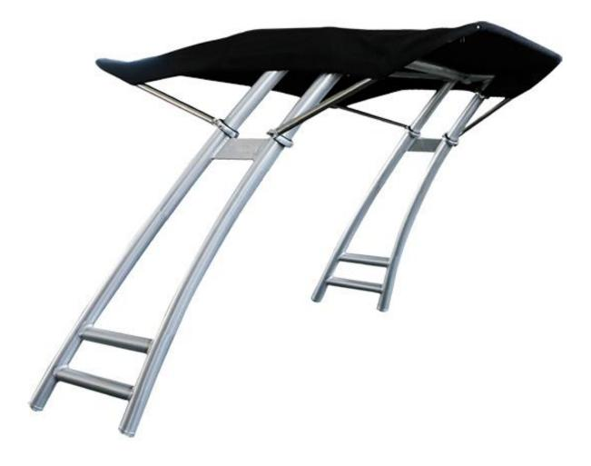
Step1: Install the clamps on the tower referring to the positions as shown in below picture. The positions of clamps are very important to ensure you get the best shape of the Bimini.
