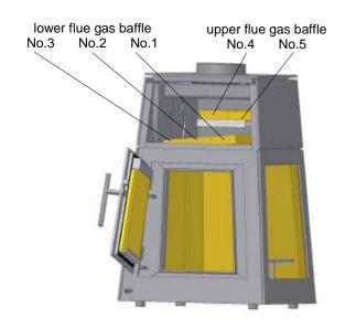
Now you can clean the plates of the flue gas baffle and insert the parts in reverse order back into the Shaker stove.
