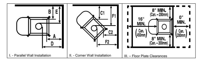
\*Note that the Parallel Wall and Corner Wall Installation clearances (diagrams I. and II.) are based on the dimensions at the top of the stove - 16" (40cm) wide x 14" (35cm) deep.
