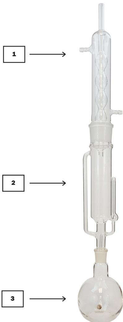
1. **Alihn Condenser** – This section of the apparatus allows for boiled solvent to condense and fall into the extraction chamber. Its side arms are for connecting to a coolant pump (not included).
