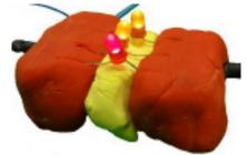
LEDs are connected to the dough each in their own circuit. Since the electricity flows through each LED independently, if one LED is removed, the others will continue to shine.
