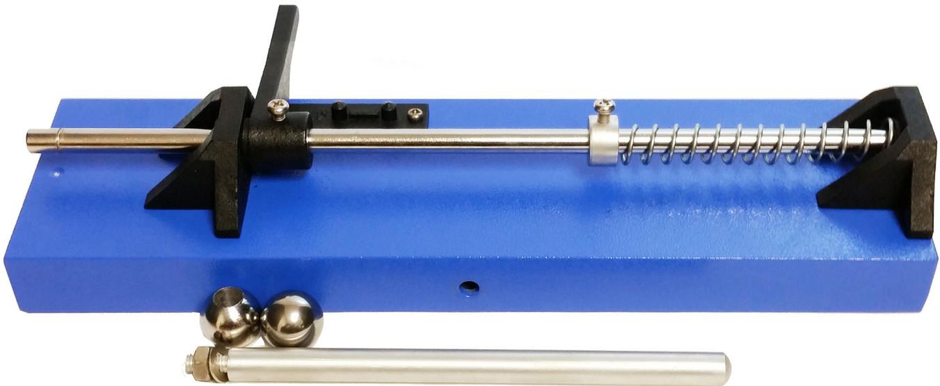
The trajectory of a solid ball projected horizontally from the front of this apparatus differs from the free falling ball drop from the rear of the unit. The difference being is the initial horizontal force imparted to the front ball. The entire concept of this piece of equipment is to prove that the two forces, horizontal and vertical, are independent of one another.
