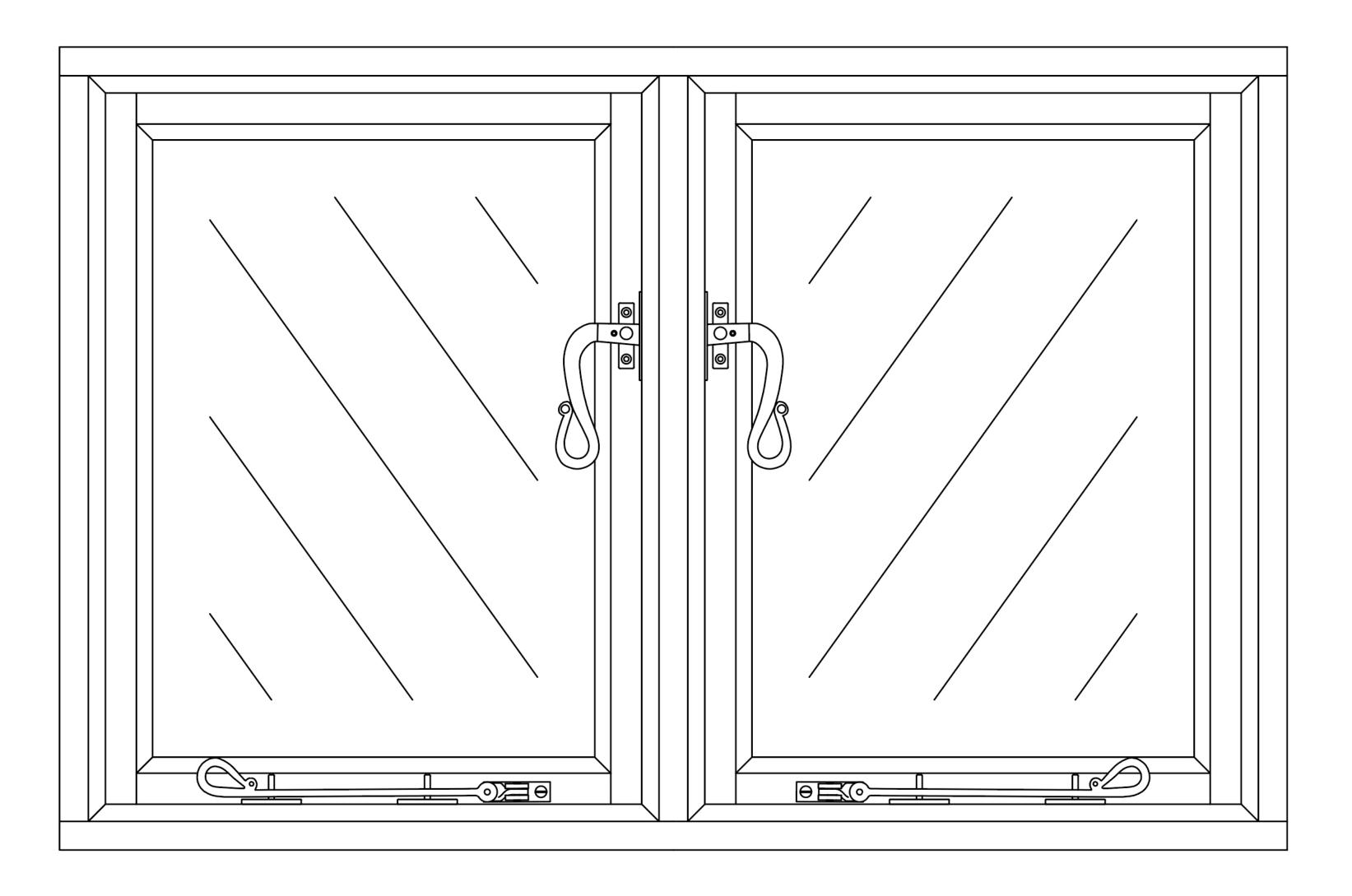
The correct casement fastener to use on a window that is hinged on the left hand side and opens away from you is the left hand casement fastener
