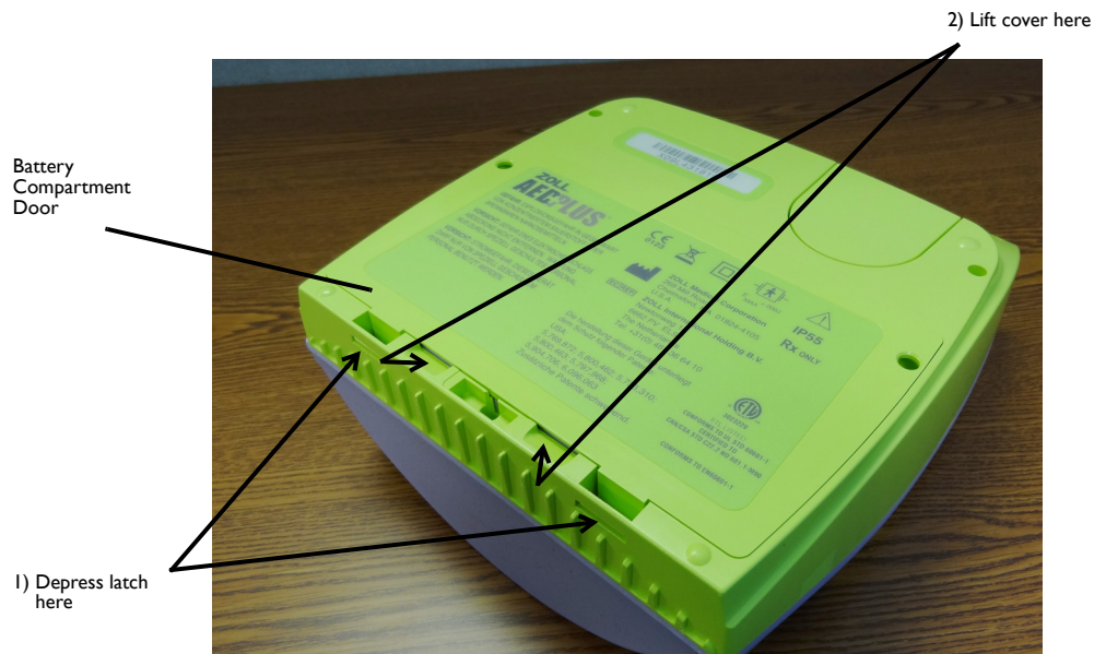
Figure 7: Removing the Battery Compartment Door
