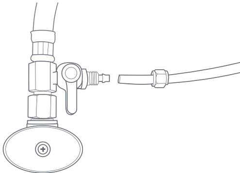
5. Screw the nut tightly into place to keep the PE Tubing securely connected to the Metal Adapter with Valve. Make sure the Valve is in the off position (perpendicular to the PE Tubing).
