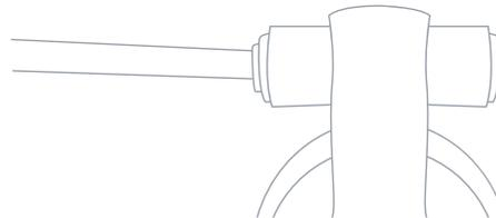
3. Hold the filter with the Filter Flushing Adapter in place over a sink. Turn the Valve of the Metal Adapter at the water source to the on position (the on position is parallel to the PE Tubing) and allow the water to flow through the Adapter and the filter for approximately 2 minutes to flush the new filter.
