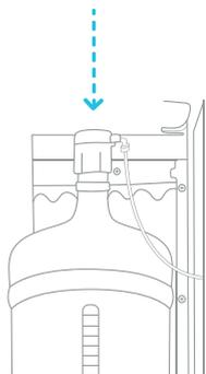
7. Slide the collar down until it clicks into place. If you are using a 3 gallon bottle rather than a 5 gallon bottle you can adjust probe by pressing the two tabs at the head of the probe and sliding the collar down to the neck of the bottle.
