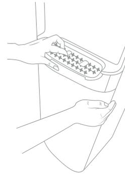
3. Gently pull the drip tray toward you to release it. Once it has been released you can remove the drip tray from the door of the cooler to empty it.
