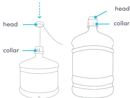
8. Push the head down until the tube hits the bottom of bottle.
