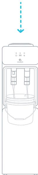
4. Place a large bucket beneath the drain outlet (#14) located on the back of the unit. Remove the drain cover and allow the water to drain from the unit. Water will start flowing as soon as the drain cover is removed.
