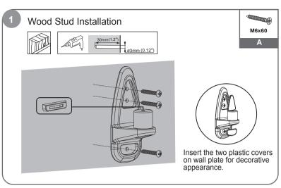
Find a wood stud In your wall and Use a pencil to mark the place for mounting. Make sure the wall structure can support the weight of monitor along with the mount. Avoid dead center for mounting holes.
