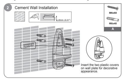
Use Cement anchors for cement walls only, Not dry wall! Pencil mark your 3 holes on concrete wall. Drill holes and insert plastic anchors. Replace mount and Screw in tightly. Test by Pulling down.
