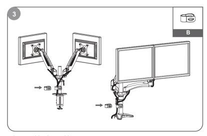
Insert cables into cable covers.
