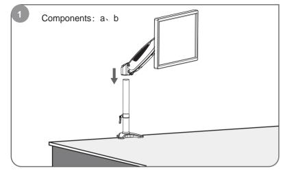
Lift the spring arm along with the monitor and put it on the steel pipe.
