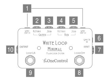
Effects connected to Loop Red and Loop Green, while being powered, can be bypassed with a true bypass switch. Effect 1 and 2 can be turned off with the Red and Green switch with one action.
