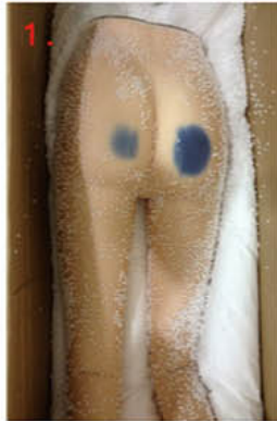
1. Stain on a pair of jeans caused by color bleeding
