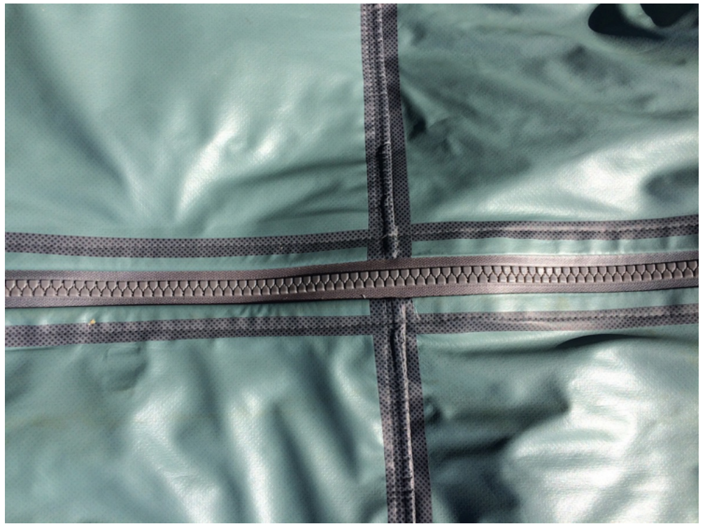
When Columbia eliminated the outer protective layer on the Reversible jacket, it had to place the waterproof seam tapes on the exterior. They are the dark lines crossing through the waterproof zipper.
