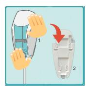
First, hold the appliance with two hands above the wall plate. Second, slide the appliance down along the front of the wall plate to capture hooks and lock into place.
