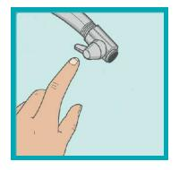
Screw the Water Diverter Valve onto the shower plumbing pipe by hand tightening.
