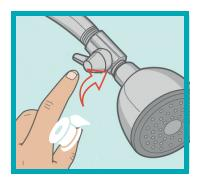
Wrap the included plumber's tape 3-4 times around the diverter valve threads in a clockwise direction prior to screwing on showerhead. Screw showerhead or handheld connector onto the Water Diverter Valve by hand tightening.
