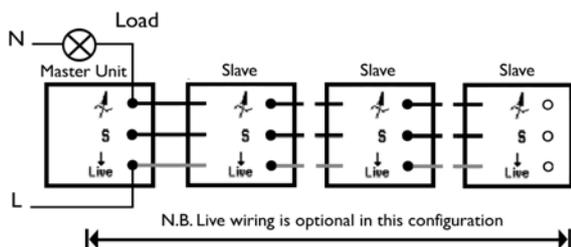
Fig 2. Wiring For Multi-Way Circuits
