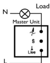
Fig 1. Wiring For 1-Way Circuits
