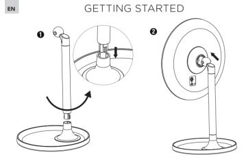
1. Assemble the stand by inserting the rod into the base. Tighten by turning anti-clockwise
