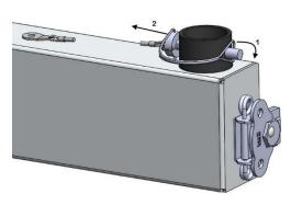
Step 4: Rotate the safety catch off the Grooming Rail's pin(1), then remove the pin (2).
