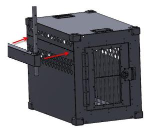
Step 6: Place Grooming Arm into Grooming Rail, and re-insert the pin removed in Step 4 through the first hole in the Grooming Arm.
