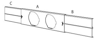
3. Open the window and place the window panel kit into the window. Adjust the extension panels B and C to fit width or height of window using the screw and nut sets mounted on the main panel A.
