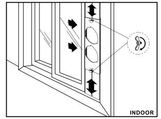
4. Insert the other end of exhaust and intake hose assembly with the hose connector to the window kit onto the window panel kit and turn counterclockwise to secure.
