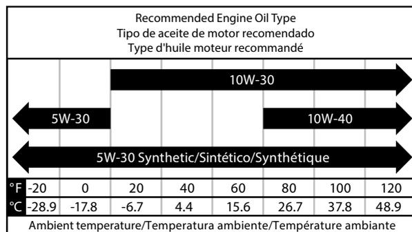
Only use 4-stroke/cycle engine oil. **NEVER USE 2-STROKE/CYCLE OIL.** Synthetic oil is an acceptable substitute for conventional oil.
