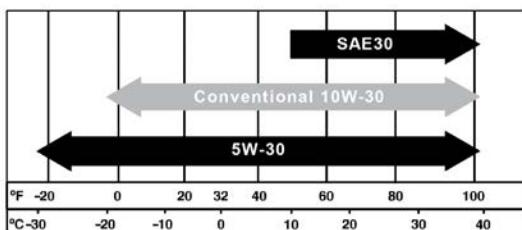
Only use 4-stroke/cycle engine oil. **NEVER USE 2-STROKE/CYCLE OIL.**
