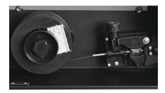
Once you are comfortable that there is a slight, even smooth drag on the welding wire spool, you may un-secure the wire from its shipping state, snip the bent end off and feed it through the spring opening on the bottom, over the drive wheel and into the torch cable. Feed it up into the cable a ways manually so it won't fall back out.
