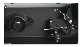
Twist the drive roller knob (4) counter clockwise to remove it. Slide out the lower drive wheel. The drive wheel will have markings on the front and back in two different sizes, in either millimeters or thousandths. A .06mm will handle 0.023 to 0.025 wire. Likewise a .08 will handle .030 wire. Be sure the correct size groove is in the outer position of the drive assembly to match the size of the wire you will be using and reinstall.
