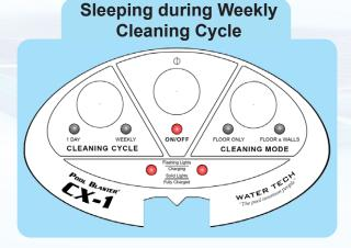
When in Weekly Sleep mode, both Cleaning Mode and Cleaning Cycle LEDs will turn off. Only the ON/OFF LED and the battery LEDs will stay on for the entire time that the robot is in sleep mode. You can leave the CX-1 in your pool while it's in sleep mode. If you take your CX-1 out of the pool, make sure you place it facing the pool so it can drive itself back in when it wakes up.
