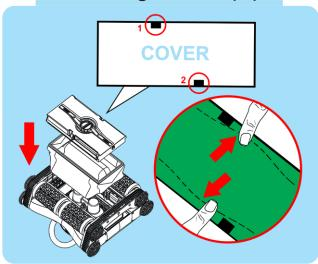
Re-insert the filter bag with the cover on top. Make sure you lock the bag under the two locking tabs (Illustrated above as #1 and #2). Then, insert bag into unit as you lower the cover into place.
