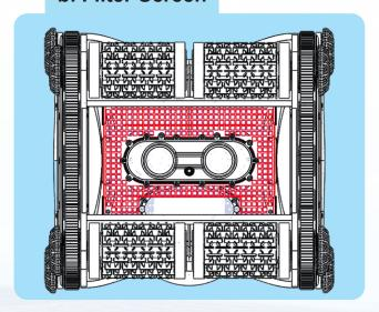
Check the filter screen (Highlighted in red above) for any debris that may have escaped the filter bag. It is recommended to occasionally clean the inside of the unit with a hose.
