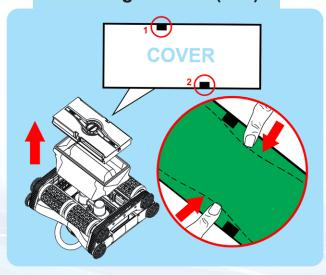
Pull out the entire bottom cover. The filter bag will be locked by the locking tabs inside the cover (Illustrated above as #1 and #2). To remove the filter bag, carefully push the filter bag out of the locking tabs.
