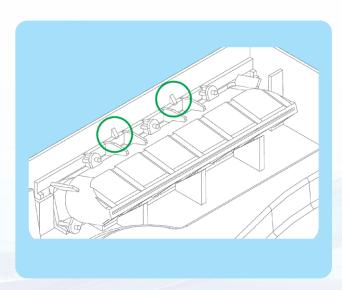
4. Press until triangular tabs snap back over valve mounts.
