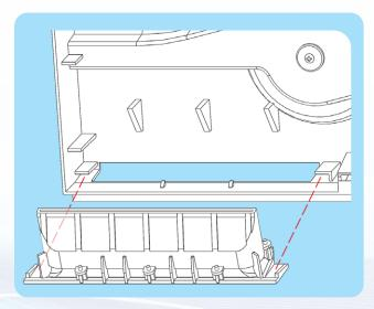
3. Align the valve mounts with the bottom cover and press down into place.
