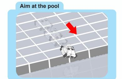
Aim the CX-1 at the pool (place robot roughly 3 ft. from the edge of the pool).
