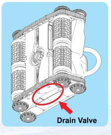
Rest the CX-1 on the edge of the pool to allow water to drain from the drain valve. Turn the power switch OFF when removing from pool, even if the batteries are fully discharged.
