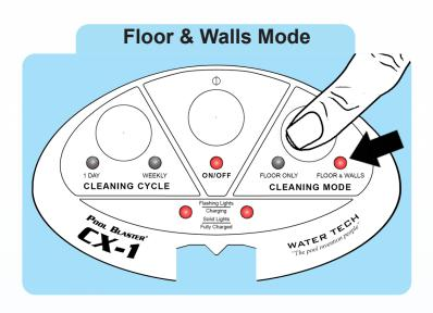
Floor & Walls – The CX-1 will clean the floors and climb the walls, enabling the CX-1 to scrub the waterline.
