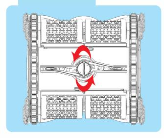
To remove the Filter Bag, flip the CX-1 upside-down and turn the knob on the bottom counter-clockwise.
