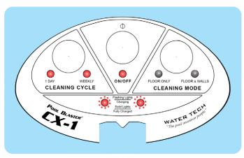
If the CX-1 is charging with the Power (ON/OFF) Button turned ON, the "1-Day", "Weekly", and "ON/OFF" LEDs will be ON (as shown on the left). The CX-1 will not be able to operate until the Power (ON/OFF) Button is turned OFF and then back ON. If you notice these LEDs are ON during charging, it is recommended that you turn the Power (ON/OFF) Button OFF.
