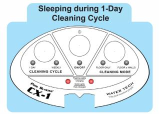
In "1-Day" Sleep mode the ON/OFF LED is off and both battery LEDs stay on. The robot will not wake from this "Sleep" mode until you turn the robot OFF and ON (or press the "Cleaning Cycle" button). It is recommended to turn the robot OFF if you do not intend on using it again immediately.
