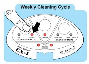
Weekly: The CX-1 will run on a schedule (illustrated on next page) that will end after 7 days, at which point the battery will be fully discharged. This mode is most effective for maintaining a clean pool as it will clean the debris that slowly accumulates throughout the week.
