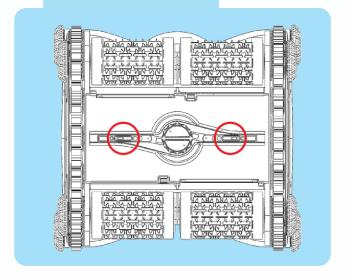
You will feel the knob "snap" as the lock is undone. Note that the locks will move inwards. This means the cover is unlocked.
