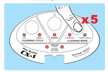
3. The "Floor Only" LED light will flash rapidly to indicate proper entry.
