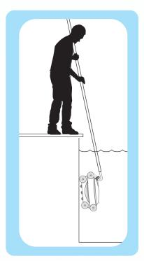
Lift the CX-1 to the surface using a slow, steady pulling motion. Remember, the CX-1 is heavy while full of water.
