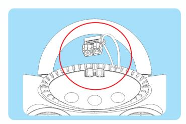
When the CX-1 is done charging, it's important that you **DO NOT** submerge the CX-1 in water without replacing the rubber plug covering the charging jack. Failure to follow this step could damage your unit.
