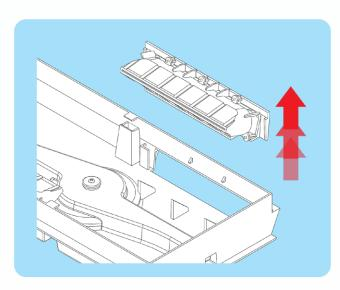
2. While still pressing outward, lift the valve mount up and out of the bottom cover. Rinse out the valve mounts and bottom cover.
