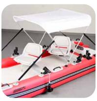
Attach the rear clips to the small D-rings behind transom. Attach front straps behind the front carry handles. Adjust and tighten straps by sliding the buckles.
