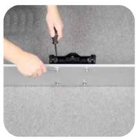
Place one washer and one nut on each screw. Tighten screw with #2 philips head screwdriver and a 7/16" or adjustable wrench. Screw must engage the nylon insert in the locking nut.
