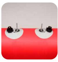
Locate seat hold down D-rings which are attached to sides of boat. Insert M6 x 50 screw with washer through each ring and fold ring flat with bolt pointing upward.
