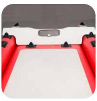
Motor Mount Transom Board Insert transom board into motor mount grommets. Plate with ring faces forward.
