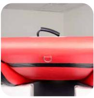
The FastCat12 has a large D-ring located under the front chamber. The D-ring can be used as an attachment point for a trailer winch or to hook up to a mooring.
