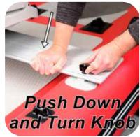
Push bench down against boat with one hand and tighten each knob.
