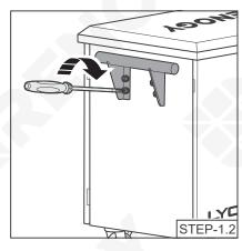
Install the Handle Bar on the left side of LYCAN with the Handle Bar Screws. Make sure that the Screws are firmly tightened with the Philips Screwdriver.
