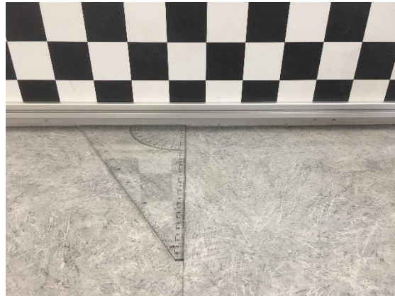
Finding a line perpendicular to the wall
