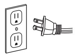
▲ WARNING: It is normal for the power cord to feel warm to the touch. However, a loose fit between the outlet and the plug may cause overheating of the plug. If this occurs, try inserting the plug into a different outlet. Contact a qualified electrician to inspect the original outlet for damage.
