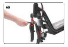
2. Remove the bolt pre-installed on the front fork arch.
