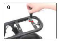
2. Remove the four bolts pre-installed on the rear rack.
