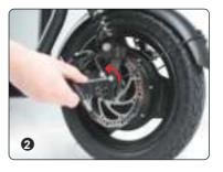
2. Remove the pre-installed bolts that secure the rear fender stay.
