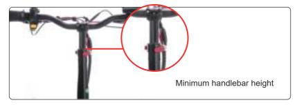
Adjust the handlebar to your desired height and then fully close the lever of the quick-release clamp.
