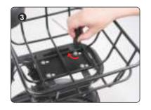
3. Align the bolt holes of the basket with thoese on the rear rack and then retighten the bolts.
