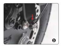
3. Pass the bolt through the hole of the rear fender stay as shown.
