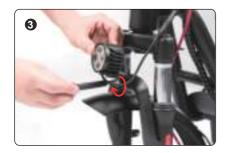
3. Pass the bolt through the front fender bracket, headlight bracket, and front fork arch. Then retighten the bolt.
