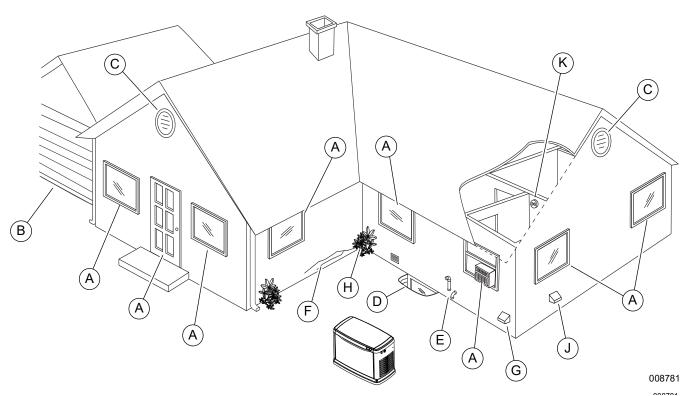
Figure 3-1. Carbon Monoxide—Potential Entry Points
