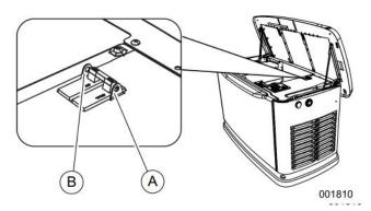
Figure 2-9. Generator Main Line Circuit Breaker
