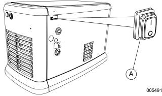
Figure 2-11. Auxiliary Shutdown Switch (all models)
