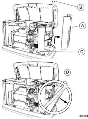
Figure 2-6. Intake Side Panel Removal
