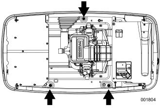
Figure 4-2. Mounting Hole Locations
