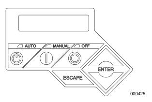
Figure 7-1. Generator Control Panel
