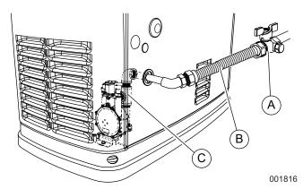
Figure 5-2. Sediment Trap, Fuel Shutoff Valve with Manometer Port, and Flexible Fuel Line
