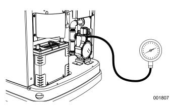
Figure 5-4. Checking Pressure with Manometer
