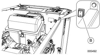
Figure 2-12. Auxiliary Shutdown Switch (14–24kW)
