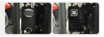
**2.** Clean foam cleaner element with cleaning solvent and blow it dry, Put a few drops of oil on the filter element;
