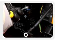
2. Attach the red clip of the special charger to the positive (red) lug of the battery, and the black clip to the negative (blue) lug of the battery. Be careful not to connect the positive and negative terminals incorrectly.
